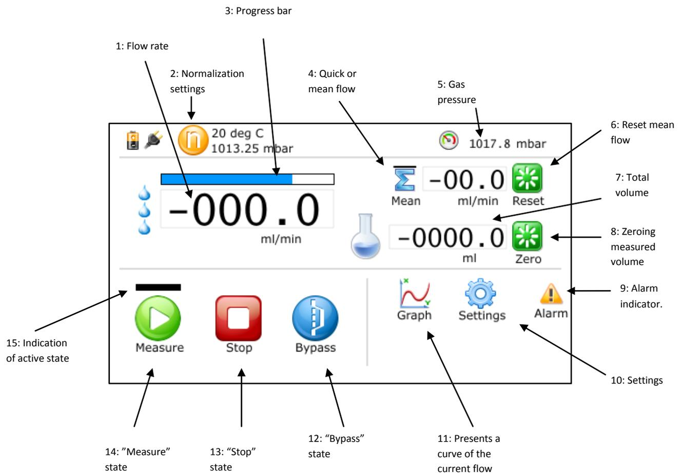
1. The flow rate is presented with the accuracy and precision stated in the specification. The update rate is dependent of the flow rate. A new flow is presented when the progress bar (3) reaches the end.
