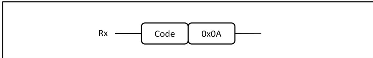
When the transmitted command request data to be returned from the ReciFlow, it will be sent directly following the echoing of the data request command code.
